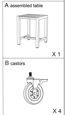
**Step 2** Lock the brake on each castor. Screw each castor into the bracket inside the leg.
